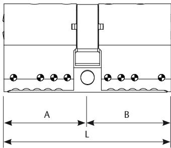
These part numbers are for modular cylinders assembled from the factory. Measurements for side A and B will be required when processing an order. The Cam, only if it is different to the standard (R15).
