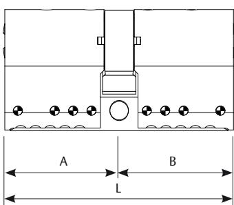
These part numbers are for modular cylinders assembled from the factory. Measurements for side A and B will be required when processing an order. The Cam, only if it is different to the standard (15 mm).
